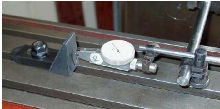
Figure 5.12 - Establishing a zero position
