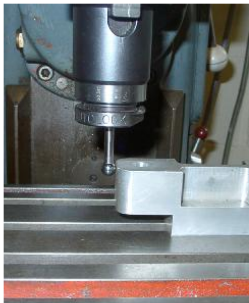
Figure 7.11 - Edge-finder in use on a mill
