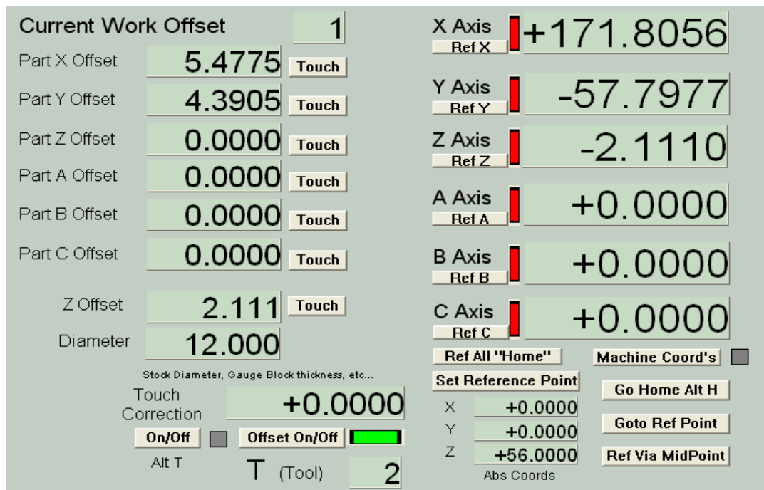
Figure 6.12 - Fixture and Tool table control family
