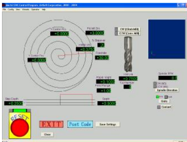
Figure 3.8 – Circular pocket with defaults
