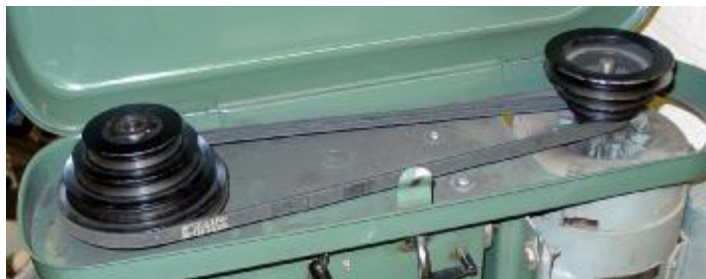
Figure 5.14 - Pulley spindle drive
